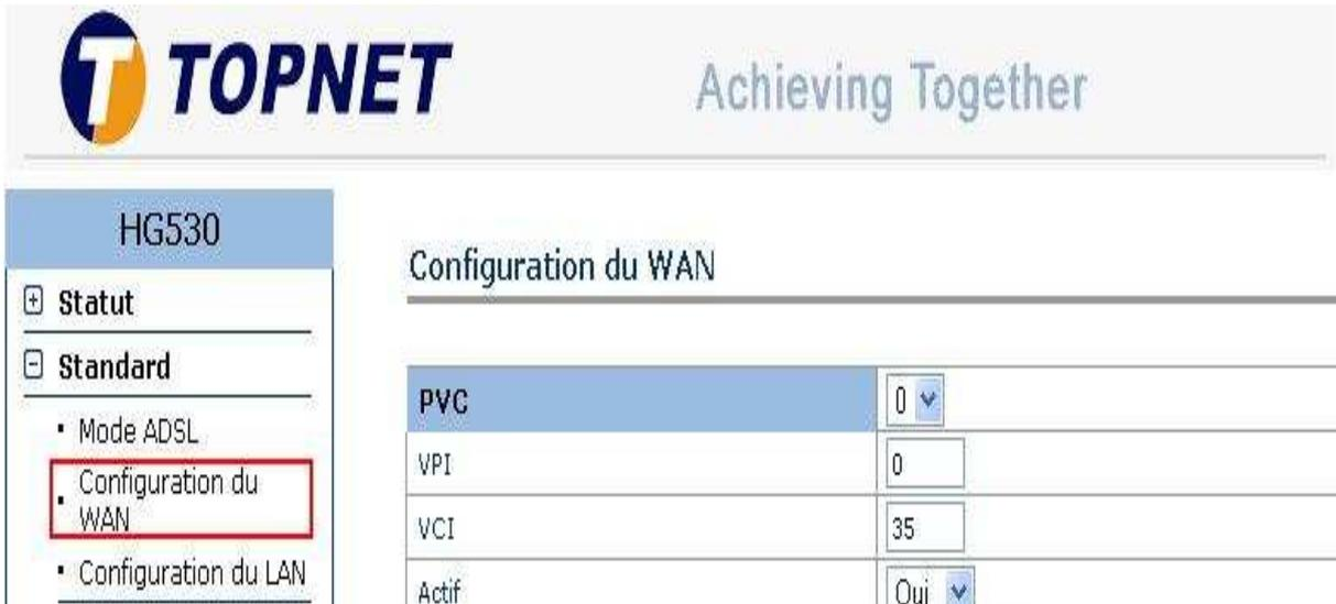
The screenshot shows the TOPNET HG530 configuration interface. On the left, a sidebar menu includes 'Statut', 'Standard', 'Mode ADSL', 'Configuration du WAN' (highlighted with a red box), and 'Configuration du LAN'. The main area is titled 'Configuration du WAN' and contains a table with the following fields:
